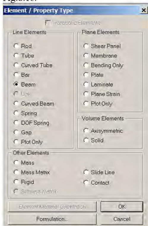
Fig.8.16. Alegerea din fereastra Element / Property Type a Element Type=Beam
